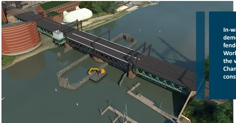
In-water construction activities will include the demolition of deteriorated portions of the existing fender system and installation of new timbers. Work will begin in the east channel and move to the west channel later in the summer months. Channel navigation will remain open throughout construction.
